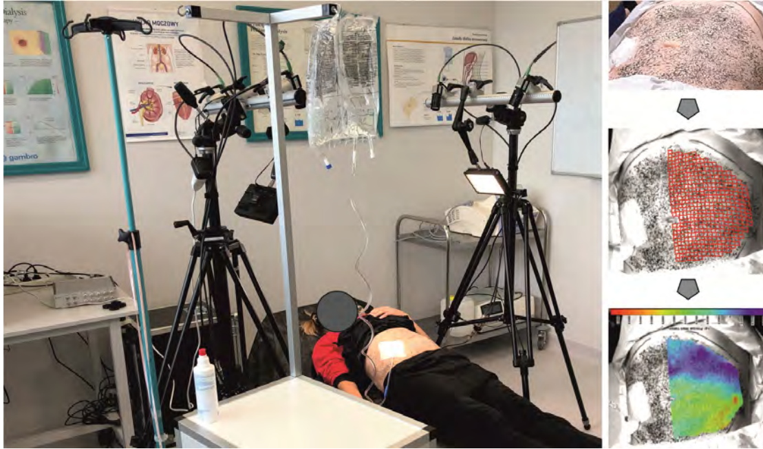
Figure 5.1: Experiment: subject laid under the DIC setup (left), speckle pattern on the surface of the abdominal wall (top right), DIC grid (middle right), and the outcome map resulting from image correlation (bottom right), Szepietowska et al. (2023) .
