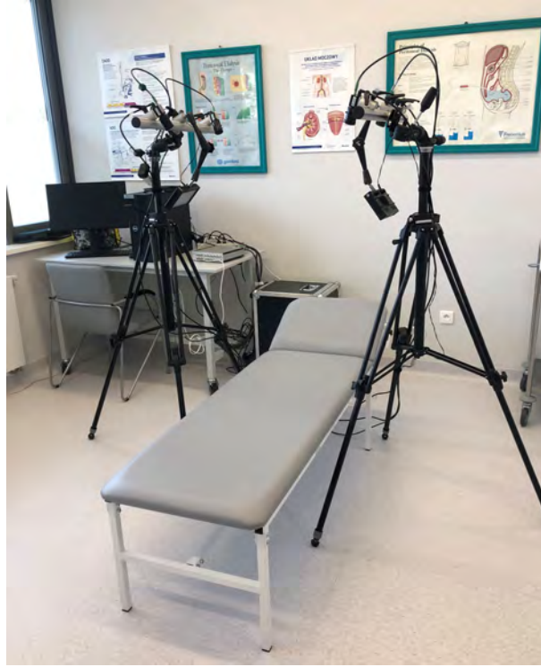
Figure 5.2: Digital Image Correlation - experimental stand, Szepietowska et al. (2023) .
